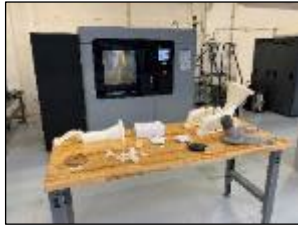
Stratasys 900MC Fused Deposition Modeling (FDM) Polymer Filament- Based Printing Large Envelope & Precise
