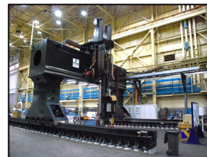
Jointless Hull Friction Stir Additive Process Worlds largest metal additive manufacturing machine. 30'x20'x12'
