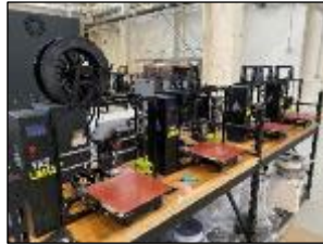
Lulzbot Taz 6 Fused Deposition Modeling (FDM) Polymer Filament- Based Printing Inexpensive, Durable, Versatile
