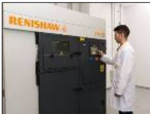
Renishaw AM500Q Laser Powderbed Fusion Powder Metal Printing Industry Standard Precision Metal Printed Parts. AISi10Mg. Aluminum Alloys.
