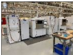
EOS M290 Laser Powderbed Fusion Powder Metal Printing Industry Standard Precision Metal Printed Parts. MS1 & 316L.
