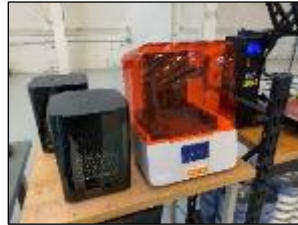
Formlabs Form 3 Stereolithography (SLA) Polymer Resin-Based Printing. Versatile Material Choices: Clear, Flexible, Durable, Medical
