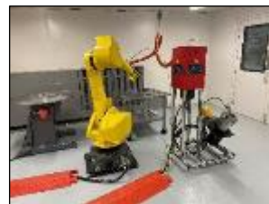
VRC Cold Spray Gas Coating Deposition Corrosion protection, repair wear surfaces, maintenance
